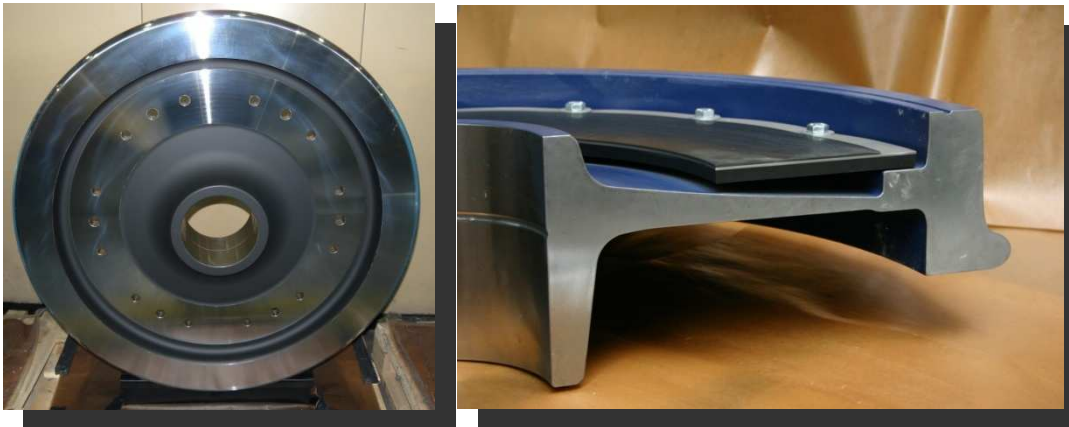
Power wheels (with noise absorbers)
